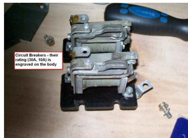
Before removing the circuit breakers make a note of the connections from each (10A, 30A) to the insulation block.
